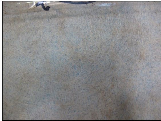
Figure 6: Same felt ply and location as shown in Figure 5, after desaturation
