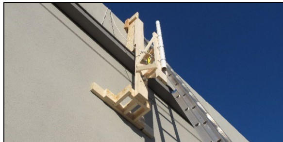
Figure 2: Dropping apparatus, setup for a 20' [6.1 m] drop height
