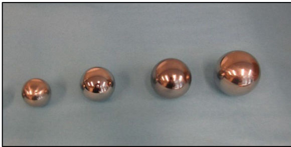
Figure 1: Steel balls used as impact strikers
