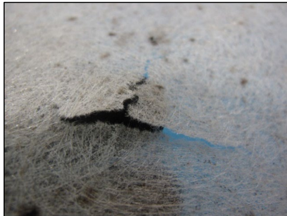
Figure 8: Same felt ply and location as shown in Figure 7, after desaturation (light pressure applied from below)
