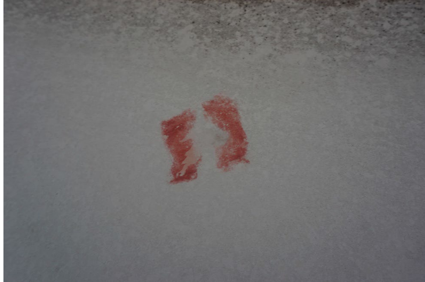
Figure 2. Burnish marks and indentation on a metal surface. The indentation is not coincident with the burnish marks, indicating that they occurred at different times.
