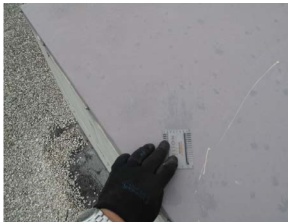
Figure 2. Burnish marks on a metal surface with a distinct directionality.
