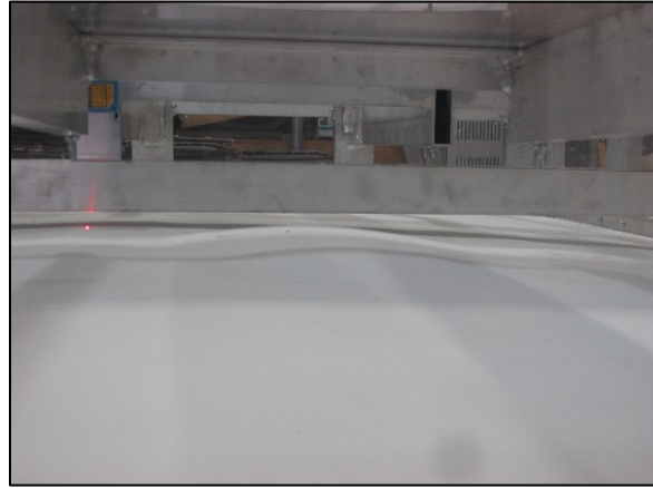
Figure 6: Expanding debonding area over a fastener location at 127.5 psf
