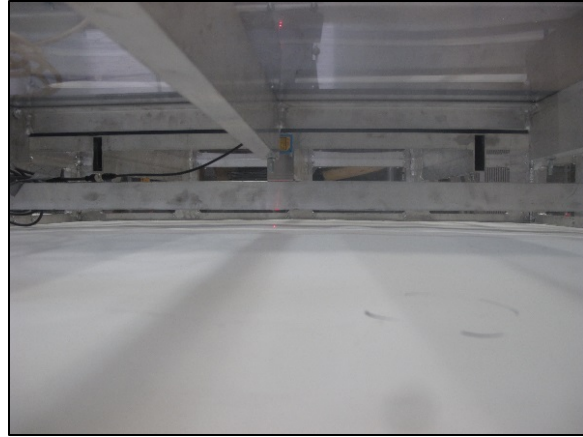
Figure 10: View across membrane for 5.0% debonded (1" diameter fractures) test at 97.5 psf uplift pressure
