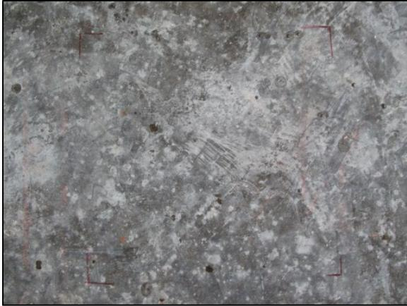
**Figure 7:** New gel formation after seven days. Note that the slab was wiped clean of gel seven days prior.
