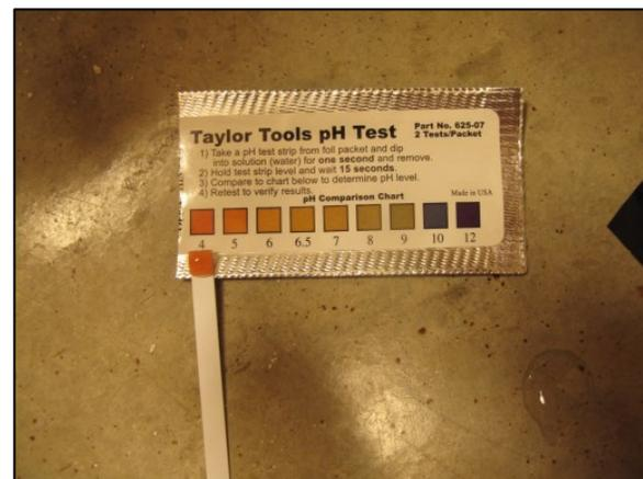
**Figure 14:** Minimal level of fluid pH at area with no gel/residue.
