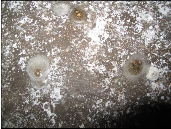
**Figure 5:** Close-up view of gel exudations and surrounding white residue.
