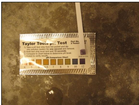
**Figure 13:** Elevated level of fluid pH at area exhibiting gel/residue.
