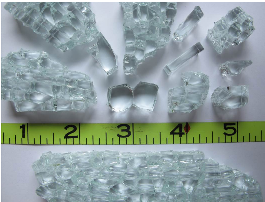
Figure 1: Recovered failure origin pieces in comparison with other pieces from a panel failure.
