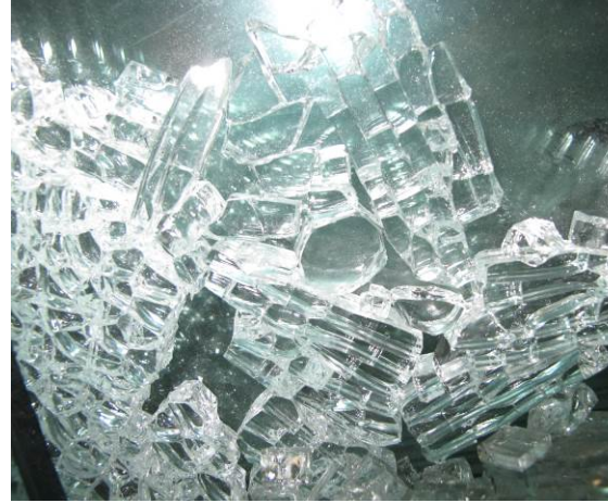
Figure 4: Detail of fracture origin piece remaining on the intact portion of the panel. Figure 5: Detail of fracture origin piece among the fallen debris.
