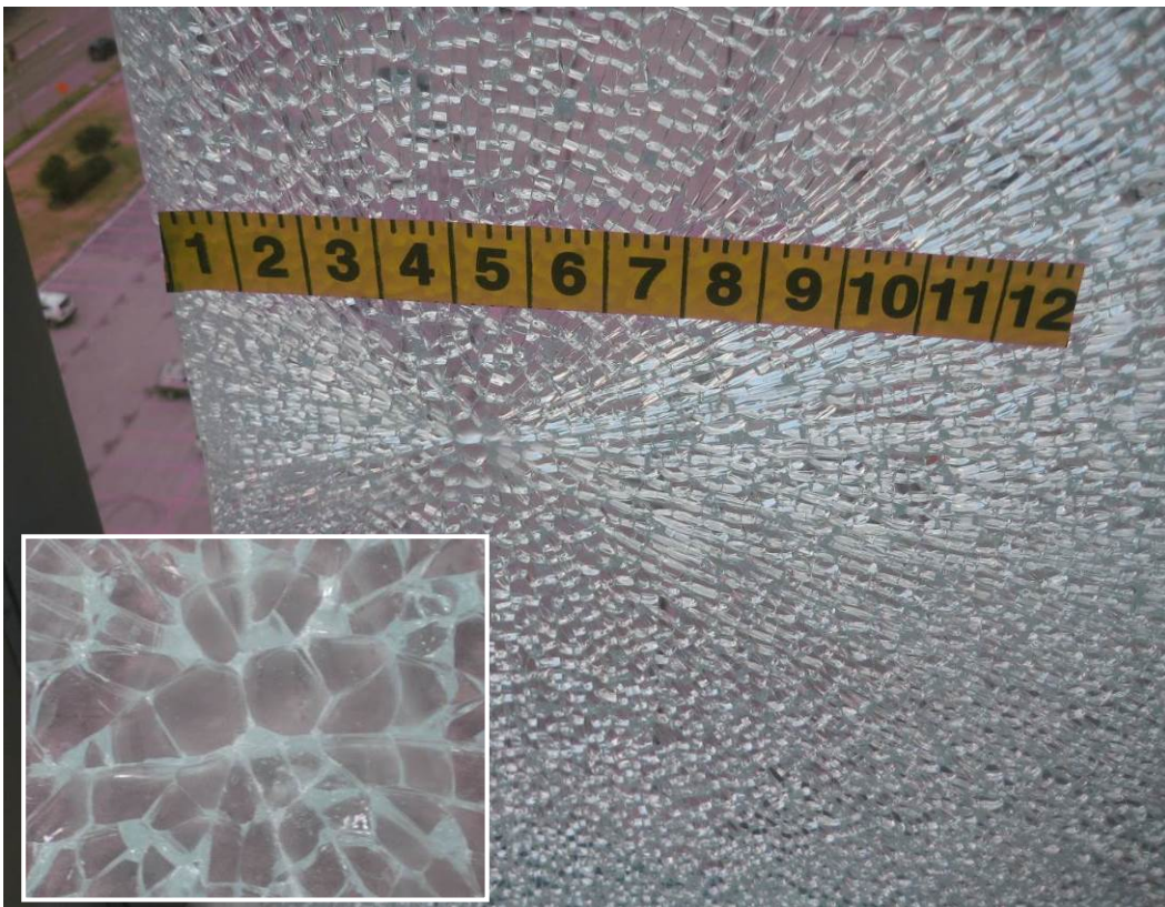
Figure 2: Fracture pattern of tempered glass panel that remained intact and detail of failure origin.
