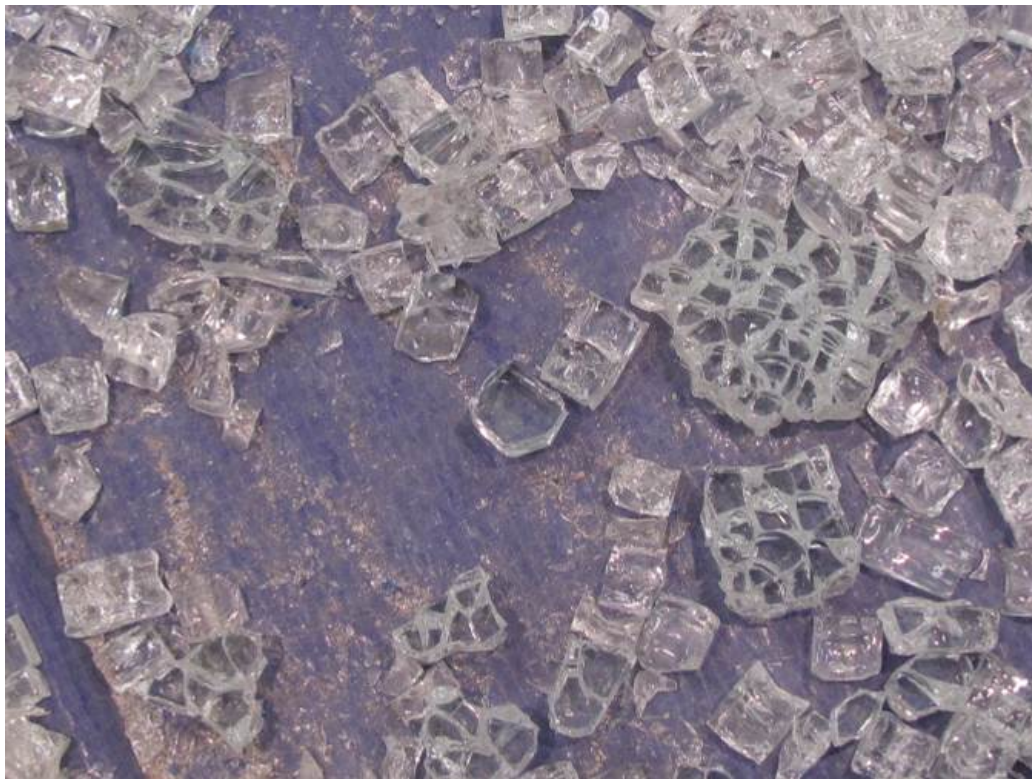
Figure 9: Closer view of previous figure. Failure origin distinct among other pieces.
