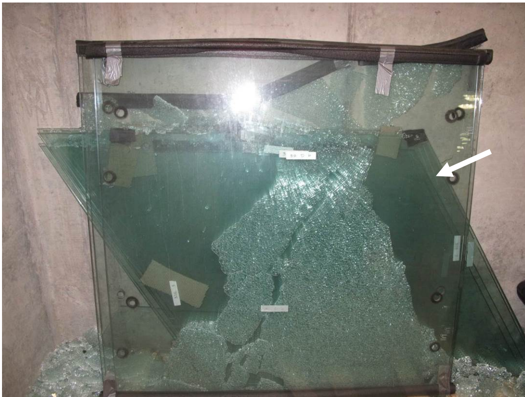
Figure 3: Partially intact tempered glass panel. Failure origin pieces are indicated.
