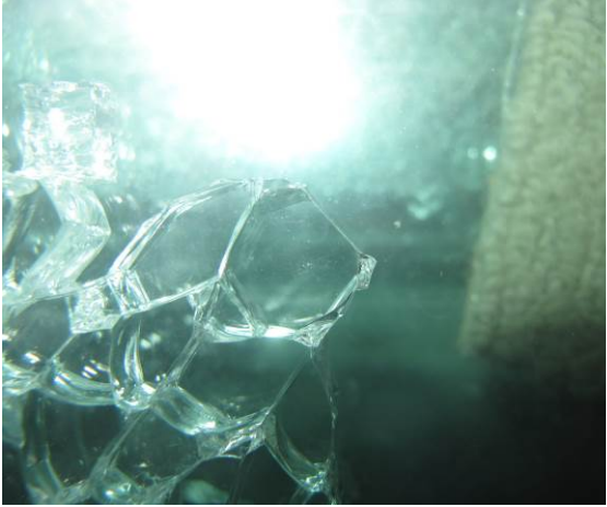
Figure 4: Detail of fracture origin piece remaining on the intact portion of the panel. Figure 5: Detail of fracture origin piece among the fallen debris.
