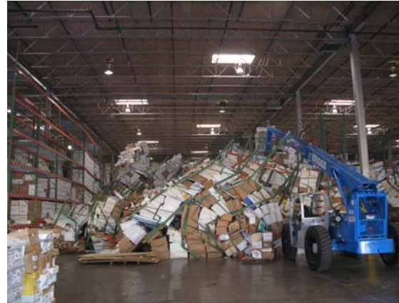
Figure 2: Collapsed Storage Racks
